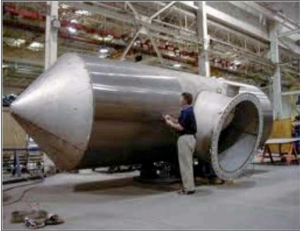
Figure 2. Examples of Wedgewire Screens for Seawater Intake
